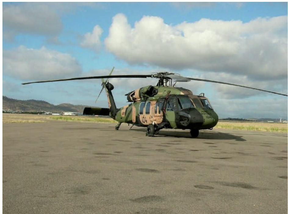
Black Hawk Helicopter from the Australian Army, Fuselage Size: 15.4 x 2.4 x 2.3 meter (Length, Width and Height)
