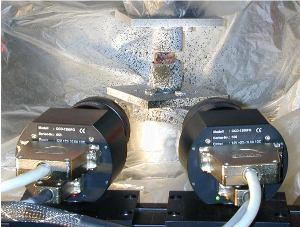
Figure 1: 3D Image Correlation camera pair on a tripod, ready for measuring of a ligament in a load frame. The ligament is prepared with a stochastically pattern; each macro facet area a separate multi-axial strain gauge. Since rigid body motion is not an issue, the same setup can be used with servo-hydraulic test machines or even in vivo.
