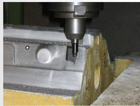
Fig. 9: Roughing in the modification area. After 30 minutes, the tool is modified.
