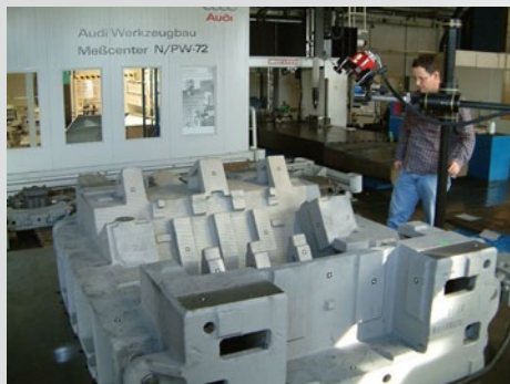
Fig. 2: Casted blank digitized using the ATOS scanner with a big measuring area
