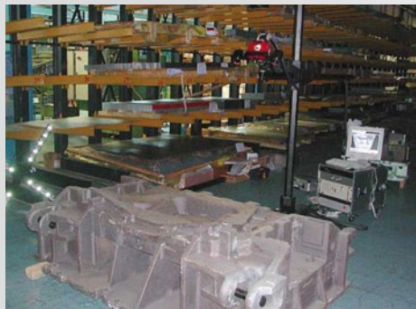
Fig. 1: Casted blank (1.5 x 1.0 x 0.5 meter) digitized using the ATOS scanner with a big measuring area
