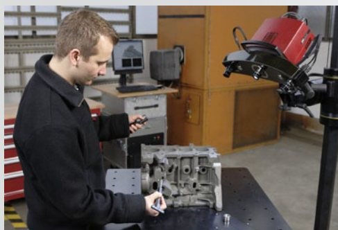
Fig. 6: ATOS System with GOM Touch Probe
