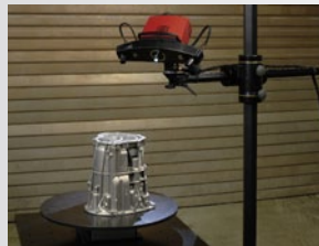
Fig. 2: ATOS Optical Measuring System for scanning casted parts
