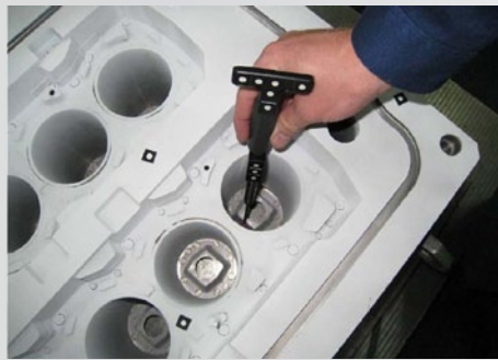
Fig. 8: Touch Probing of deep cylinder
