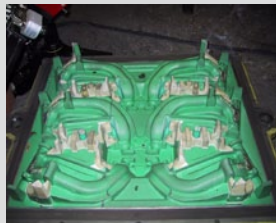
Fig. 1: Measurement of a Pattern Plate with ATOS System
