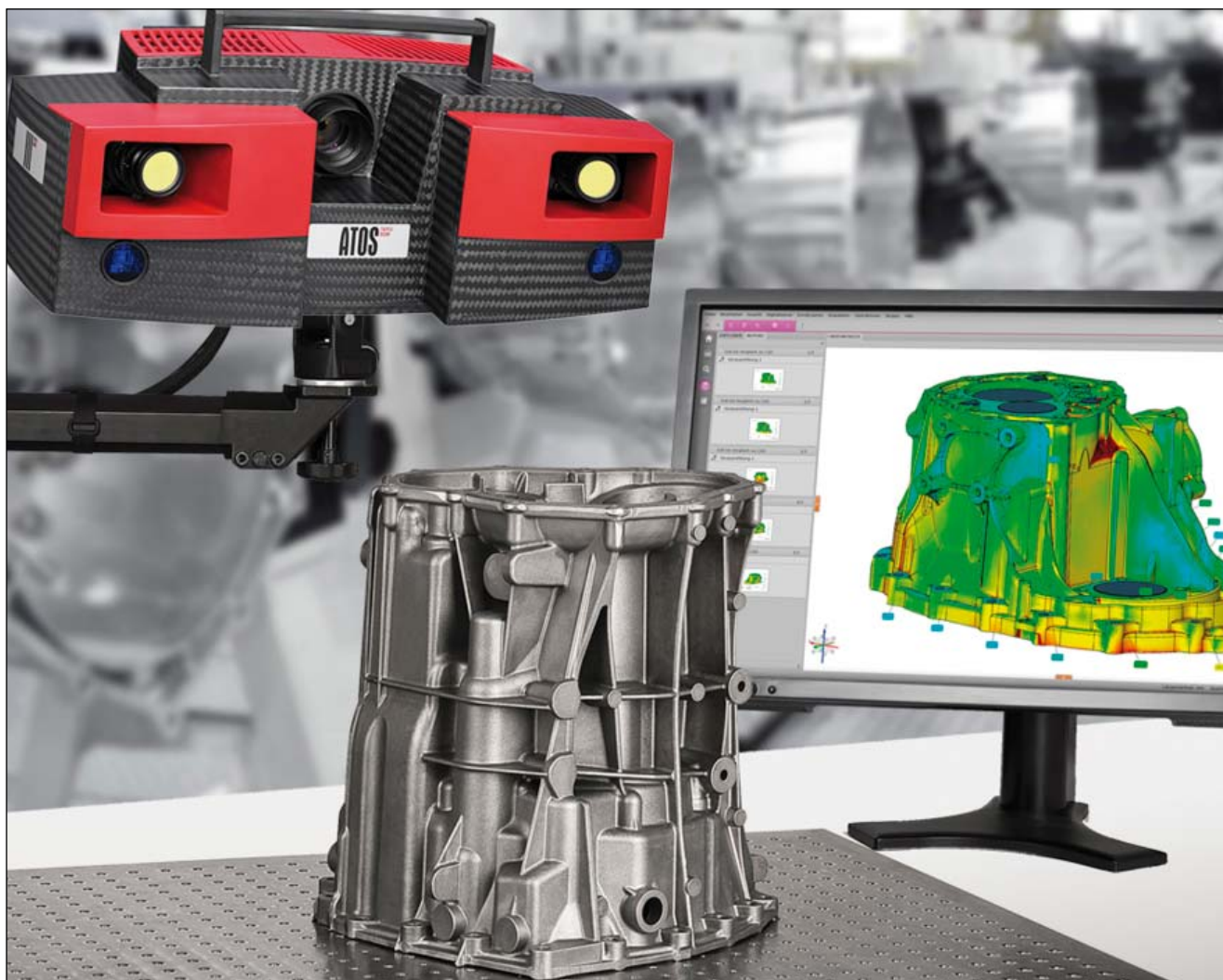
Atos triple scan 3-D coordinate measuring system for complete surface measurement of castings (Photos: GOM)
