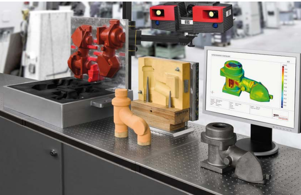
Figure 2: Optical measurement supports and speeds up virtually all processes from pattern and tool making via mold and core making through to first article inspection (FAI) and optimization of CNC machining
