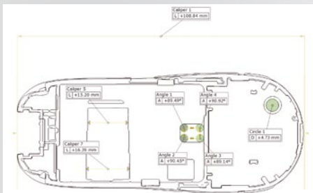
Fig. 5: 2D analysis with the ATOS CMM inspection tool
