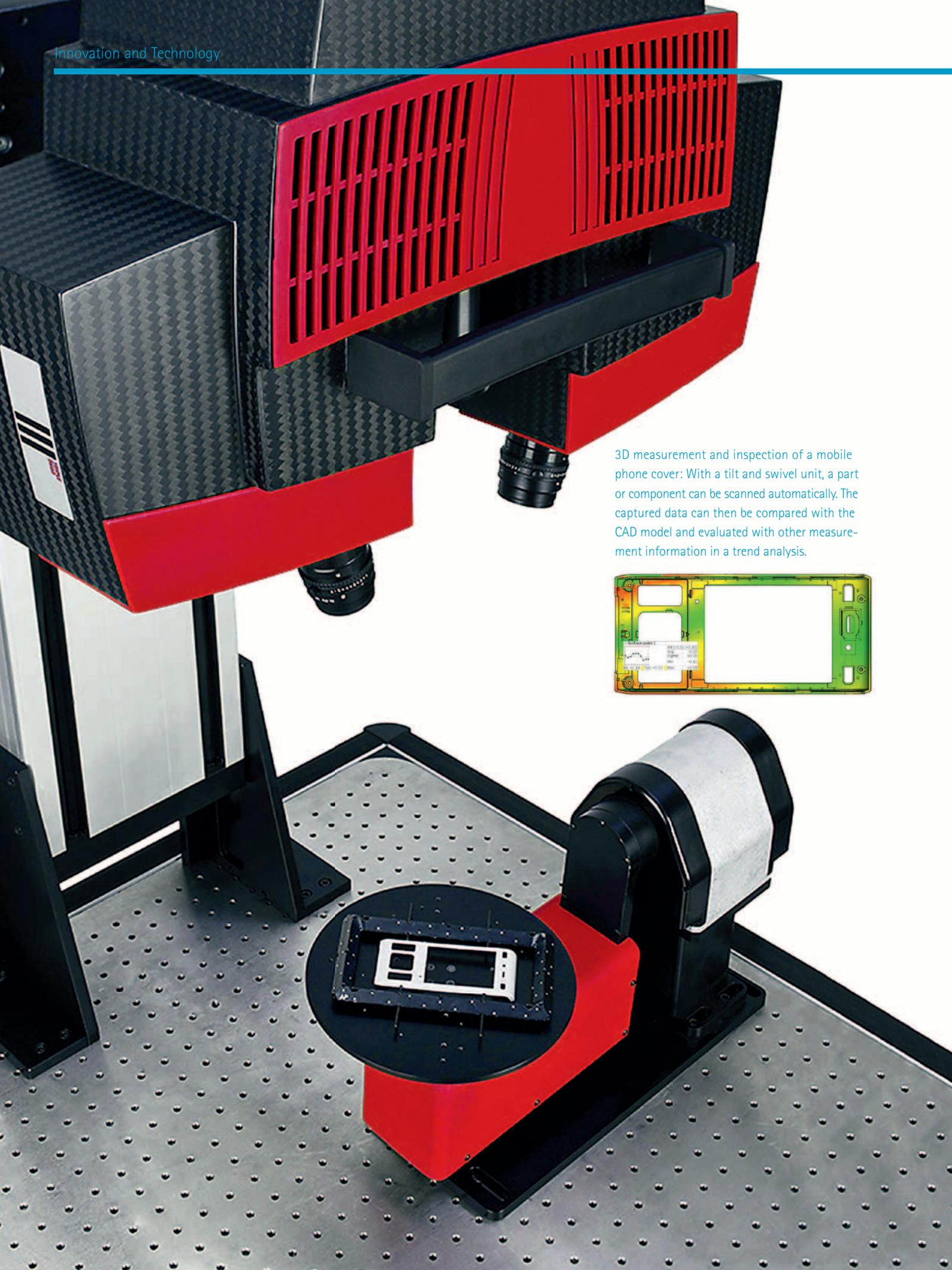
3D measurement and inspection of a mobile phone cover: With a tilt and swivel unit, a part or component can be scanned automatically. The captured data can then be compared with the CAD model and evaluated with other measurement information in a trend analysis.
