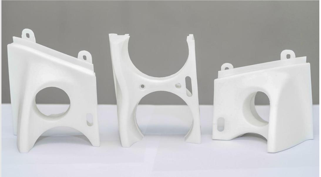
Finally the parts were chemically welded together using acetone. The gauges were temporarily installed to ensure that the part was geometrically accurate.
