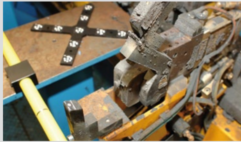
Fig. 2: Detail view of a clamping fixture to fix the sheet metals. The reference point on the bearing area is visible.
