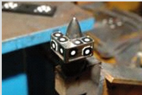
Fig. 3b: Detail view of reference points: cylinder adapter with magnetically fixed on the adjustment pin
