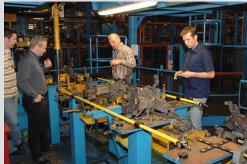
Fig. 1: Welding fixture of a side panel before measuring in the production environment (with Invar scale bars and orientation crosses)
