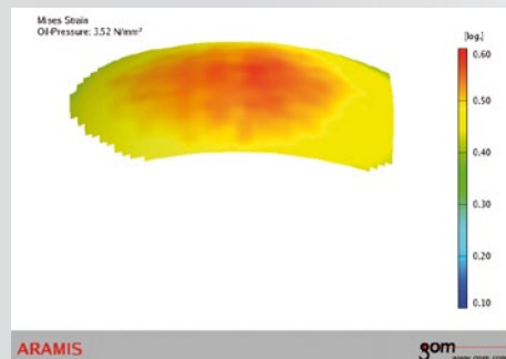
Fig. 13: Shape of the sheet metal specimen with visualization of the equivalent total strain acc. to von Mises.
