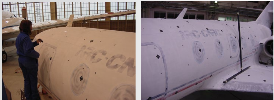
Fig. 3: Shown is the application of the markers on the plane.
