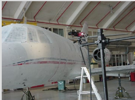
Fig. 5: Digitizing of the object using the ATOS II system
