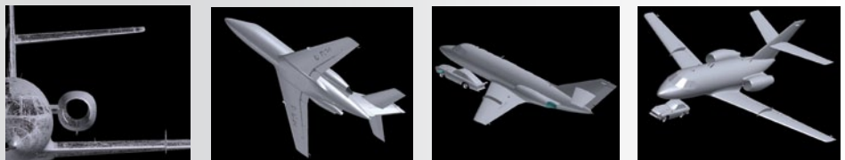
Fig. 10: Shown are different views of the gathered data, in the both right images in comparison to a digitized real size car. ATOS XL is proven for car manufacturers and is increasingly used also for much bigger objects, if dense and high accurate data is needed.
