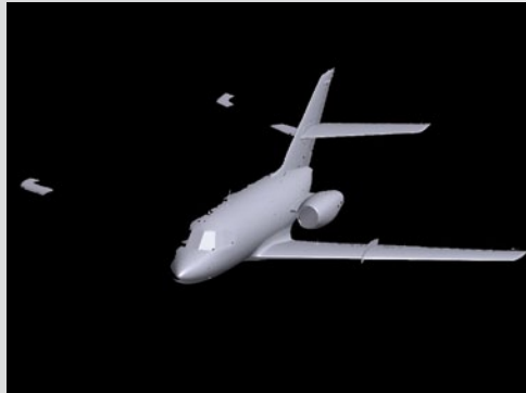
Fig. 8: Wing tip data to check for symmetry and allow an accurate mirroring to create a full aero model.
