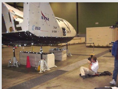
Fig. 4: TRITOP CM M measurement
